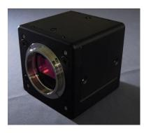
BV-C3201 is a line scan camera using prism optics and two InGaAs line sensors and as it outputs each image alternately, the line rate is doubled. Two image sensors are the same and each is 512 pixels.
