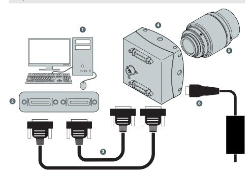
Fig.: 4-3: Connecting camera and image processing system
