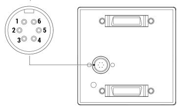
Fig.: 4-1: Power connector pinning
