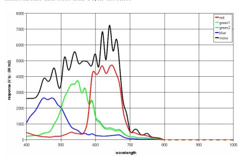
Fig.: 5-3: Quantum Efficiency mono and color with UV/IR Cut Filter
