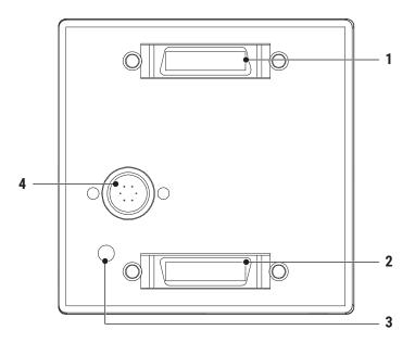
Fig.: 3-1: Interfaces of the camera EoSens® CL
