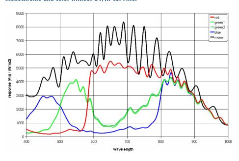
Fig.: 5-4: Quantum Efficiency mono and color without UV/IR Cut Filter
