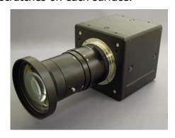
BV-C3350 uses a beam splitter and two line sensors which each sensor has different focal points. Therefore, BV-C3350 can get two images with the different focal points at the same time and with the same field of view. This function will be convenient for a glass cover investigation on surface and inside, for instance.
