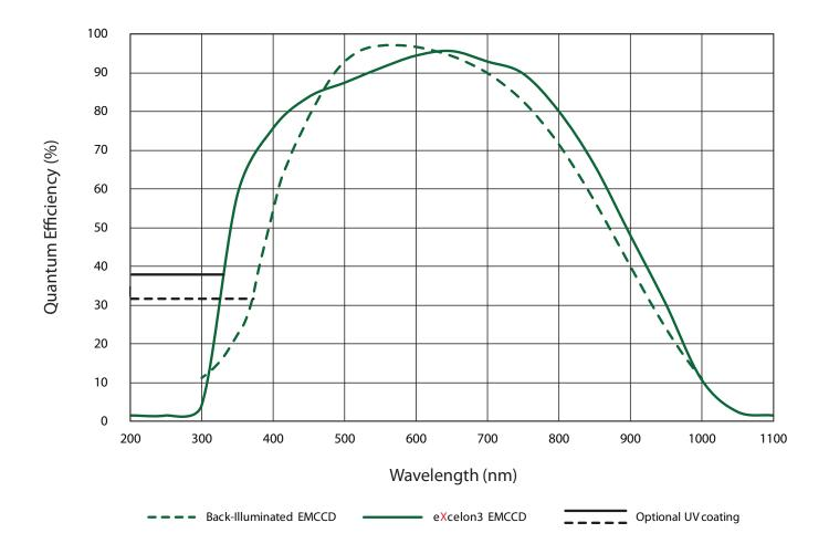
NOTE: Graph shows typical Quantum Efficiency (QE) data measured at + 25°C, representing expected performance at this temperature. QE will be lower at operating temperature. For the best results for your application, please discuss the specific parameters of your experiment with your sales representative.
