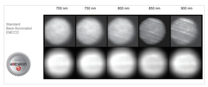
Data taken with white light source through a monochromator comparing etaloning performance of eXcelon vs conventional back-illuminated EMCCDs.
