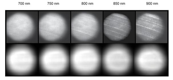
Data taken with white light source through a monochromator comparing fringe supression of eXcelon vs. conventional back-illuminated EMCCDs.
