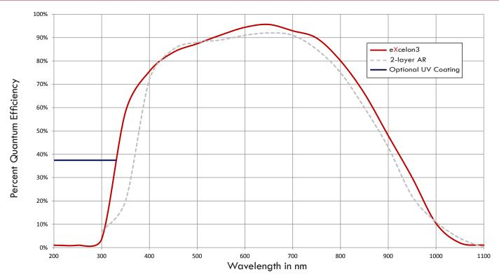
NOTE: Graph shows typical Quantum Efficiency (QE) data measured at + 25° C. Quantum Efficiency is a function of temperature and actual results will depend upon CCD temperature.
