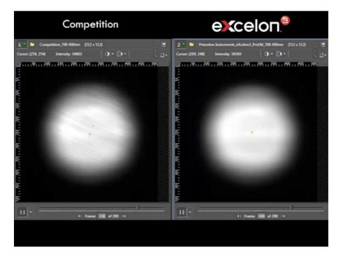
Image shows the reduction in etaloning provided by eXcelon3 back-illuminated EMCCDs (right) compared to less-sophisticated back-illuminated EMCCD designs (left).
