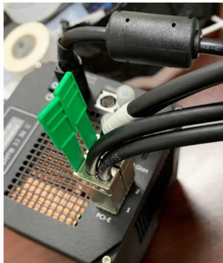
PCIe cables inserted into camera's PCIe ports.
