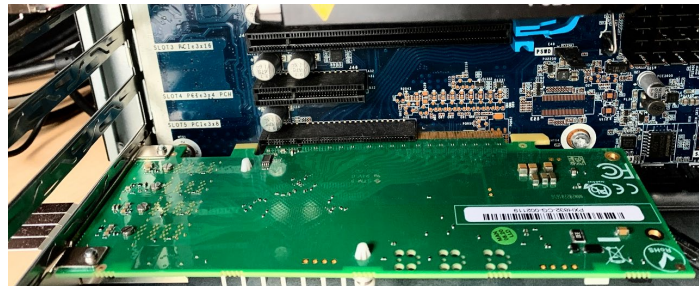
PCIe card inserted into an 8-channel PCIe slot. Note the remaining free-floating PCIe slots.
