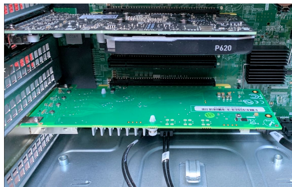
PCIe card inserted into a 16-channel PCIe slot.
