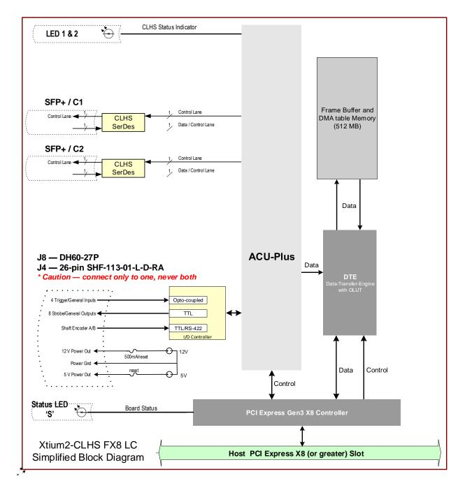
Figure 10: Xtium2-CLHS FX8 LC Block Diagram
