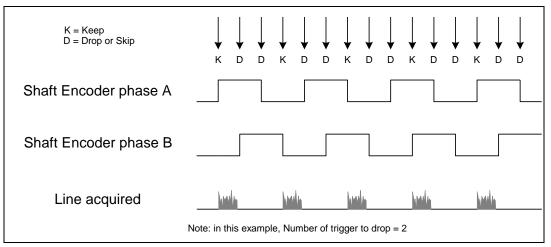
Figure 13: Encoder Input with Pulse-drop Counter
