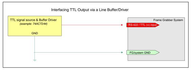
Figure 35: Interfacing TTL to TTL Shaft Encoder Inputs
