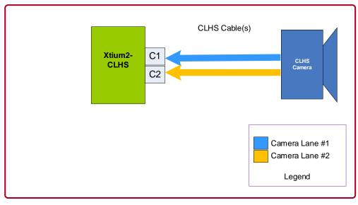
Figure 23: One Camera up to 2 lanes Block Diagram
