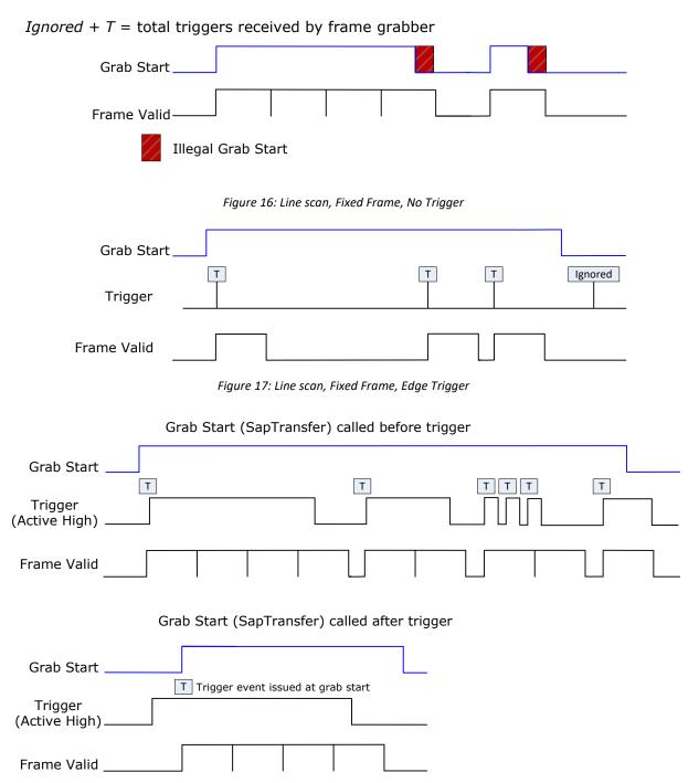
Figure 18: Line scan, Fixed Frame, Level Trigger (Roll-Over to Next Frame)
