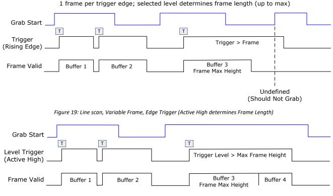
Figure 20: Line scan, Fixed Frame, Level Trigger (Roll-Over)
