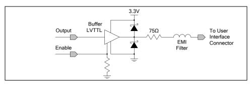
Figure 29: General Outputs Electrical Diagram
