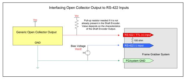
Figure 34: Interfacing to an Open Collector Output
