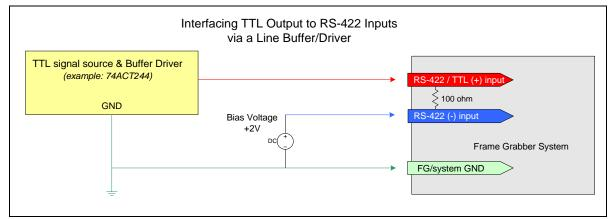
Figure 36: Interfacing TTL to RS-422 Shaft Encoder Inputs using a Bias Voltage
