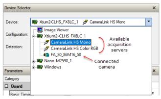
The Xtium2-CLHS FX8 LC firmware supports multiple configurations that include support for single or multiple Camera Link HS cameras and provides the following acquisition servers:
