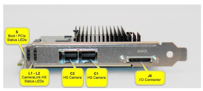
Figure 22: End Bracket Details
