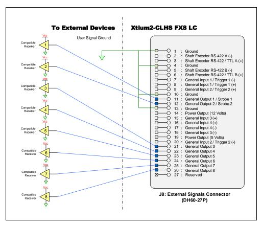
Figure 30:Output Signals Connection Diagram
