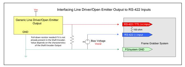
Figure 33: Interfacing to a Line Driver Output
