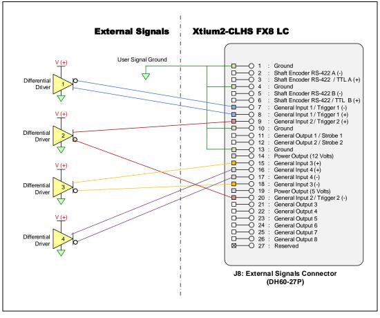
Figure 28:External Signals Connection Diagram
