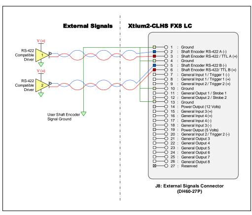
Figure 32: External RS-422 Signals Connection Diagram
