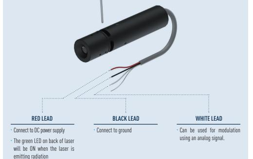
**Clamping area =** For optimal performance and lifetime of the laser, fixing the laser using a C-mount bracket (or any bracket with increased contact area) is recommended. The designated clamping area of the laser can be found on the mechanical drawing in the Datasheet.
