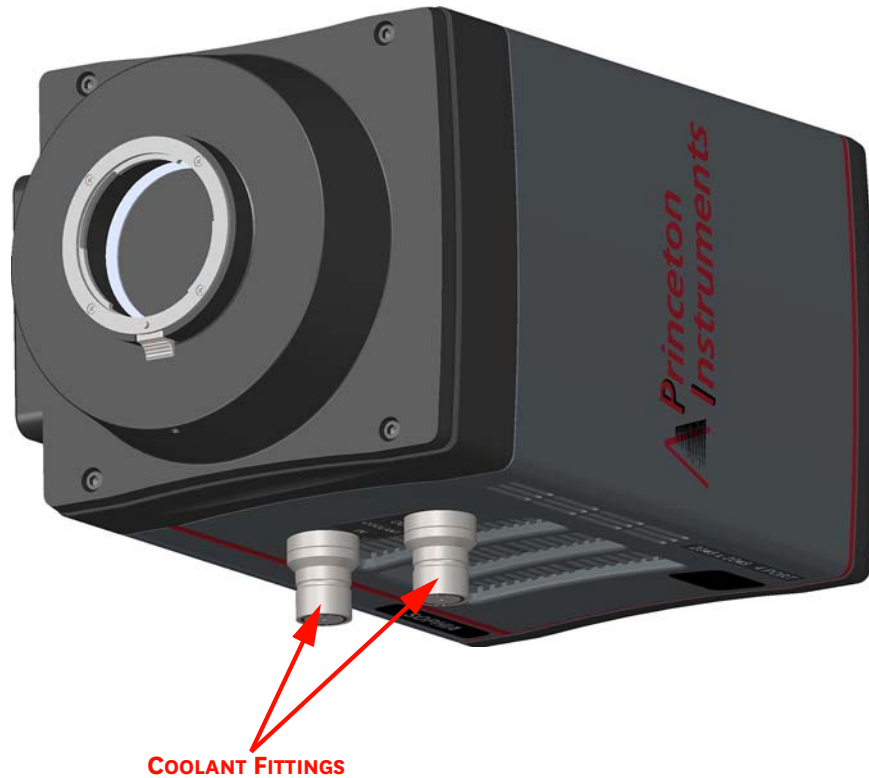
Figure C-1: Positioning SOPHIA to Drain Coolant
